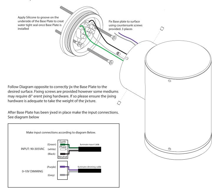
Once Wall preparations and input connections are completed. Slide the base and head over base plate. Once in position ÿx in place using the three grub screws.
