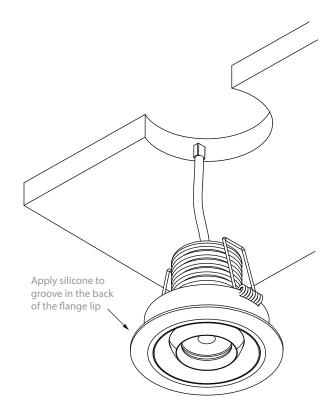
Draw power supply cable down through the cut hole and make a good electrical connection with the fixture input cables. See diagram for correct wiring. Be sure to leave extra length to allow the fixture to be removed from the ceiling without disconnection for servicing.
